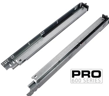
Type: Soft-Close, Full Extension Concealed Undermount Slides Weight Rating: 100 lbs. Dynamic Material: Cold Rolled Steel Hole Pattern: 32mm Finish: Zinc Industry Rated: BHMA, KCMA, BIFMA, ANSI
