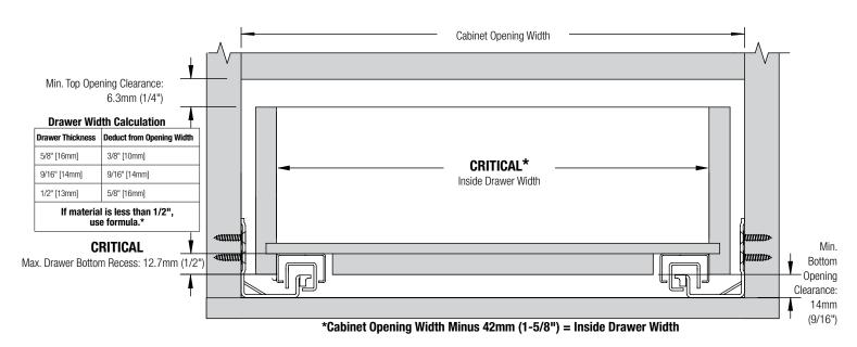
MuV+ Maximum Drawer Side Material Thickness: 16mm (5/8") Use Muv+34 for Drawer Material from 16mm (5/8") to 19mm (3/4")
