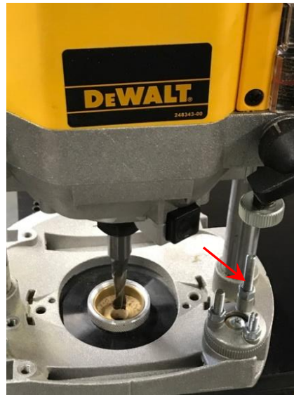
Long stop/shallow cut (3 mm) with stop bar pulled out as shown in Fig. 13.
